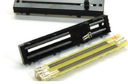
Smooth 60mm slide input faders or high-precision mixing.
