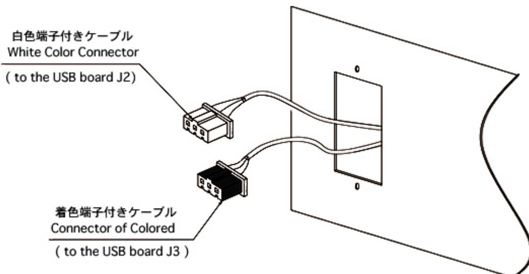
3. When you can verify that you connect to the J2 terminal and the J3 terminal just, in order in the type where the TUB-1 installation hole becomes depth for the LED indicator lamp to be above, it inserts in the installation hole, it locks with bis 2 you remove some time ago. In addition, when it is the type where the TUB-1 installation hole becomes wide, in order for the LED indicator lamp to be left side, please install.
