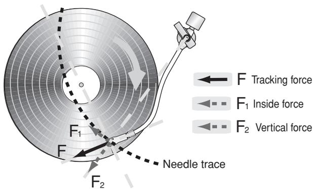
The tracking force (frictional force) generated between the stylus and the record disc makes the inside force.
